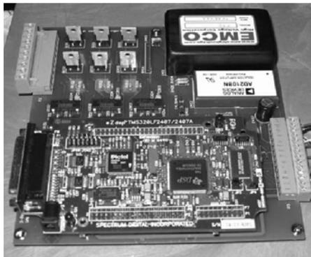
Fig. 8 Digital Signal Controller and Complementary Circuitry
