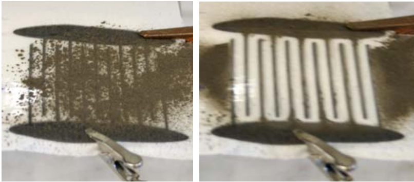
Fig. 9. Before and after photographs of a dust shield on fabric with JSC-1A lunar simulant.
