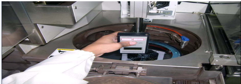
Figure 3: A photo showing the method of verifying the static voltage accumulated on wafer saw using electrostatic field-meter.
