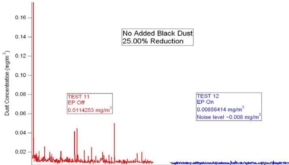
Fig. 8. The TSI DustTrak measured concentrations of as-delivered GN<sub>2</sub> with the precipitator off (red) and the precipitator on (blue). Each measurement was performed over a 10 minute period.
