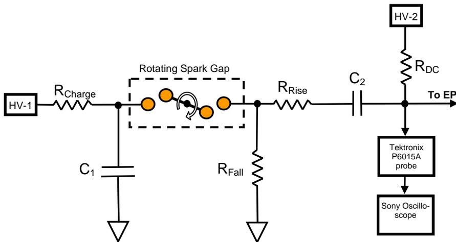
Fig. 5. Wiring schematic of the pulsed power supply used for the EP.
