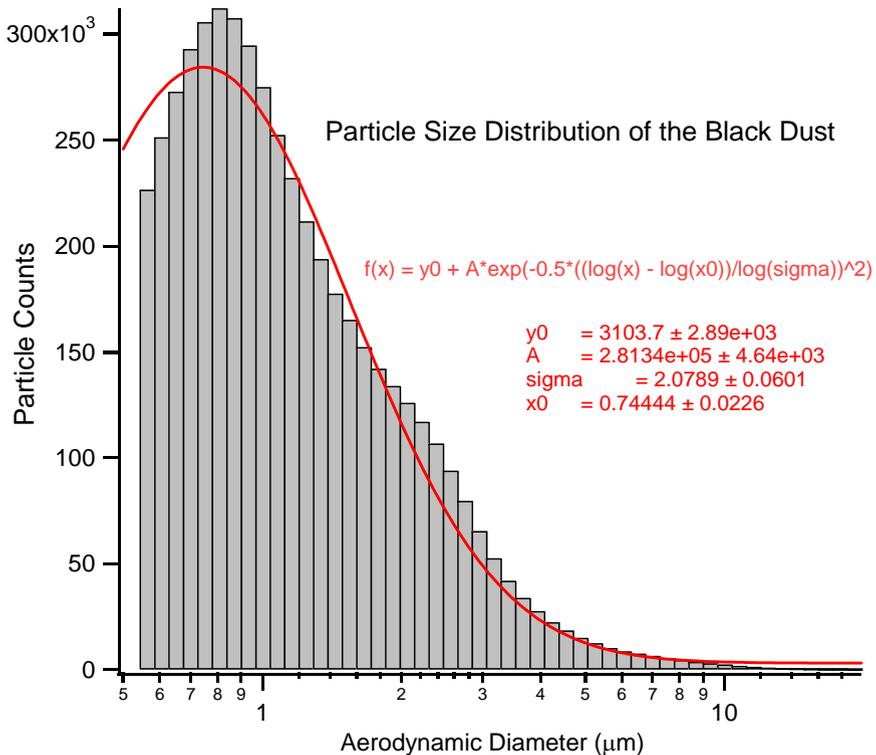
Fig. 2. The log-normal distribution of the black dust along with the fitting parameters used to generate the fit (red line).
