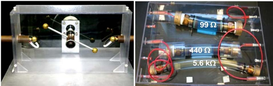
Fig. 6. Pictures of the (left) Rotating Spark Gap and (right) liquid resistors used for the pulsed power supply.
