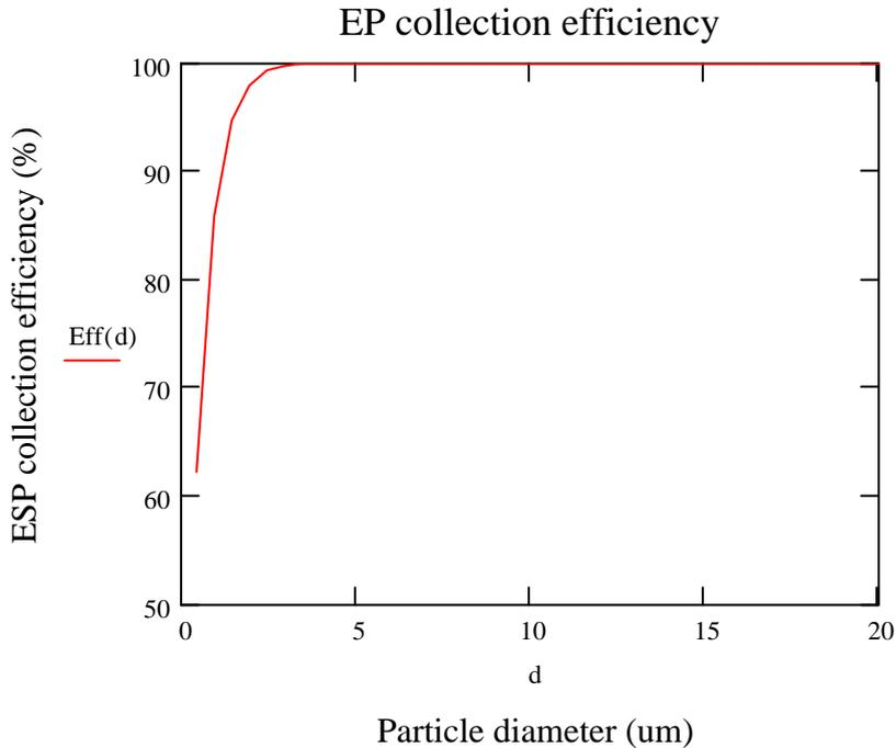
Fig. 3. The EP efficiency as a function of particle size.
