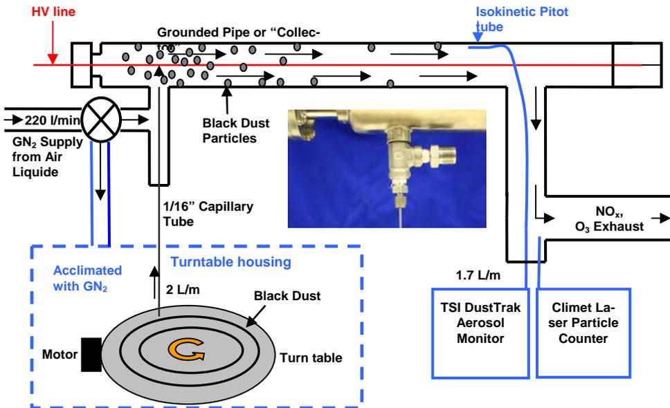
Fig. 4. Air flow schematic of the EP demonstrating how the capillary tube is used to transfer the dust from the turn table to the EP. At the end of the EP an isokinetic Pitot tube samples the dust flow concentration measured by a TSI DustTrak Aerosol Monitor and a Climet model CL-150t Laser Particle Counter.
