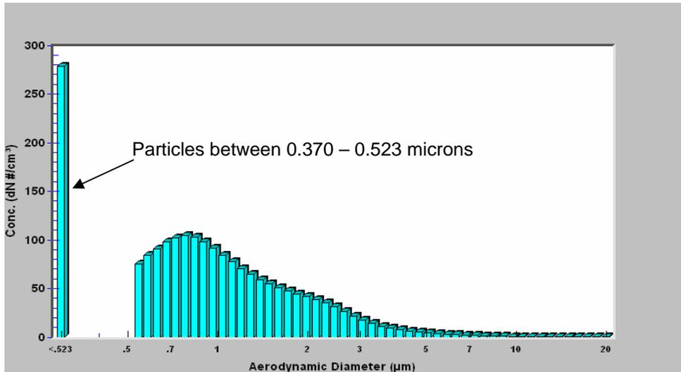
Fig. 1. Measurements of the PSD of black dust using the TSI Model 3321 Aerodynamic Particle Sizer.
