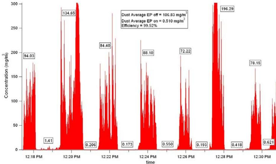
Fig. 9. A sample data set of the measured black dust concentrations turning the precipitator on and off.
