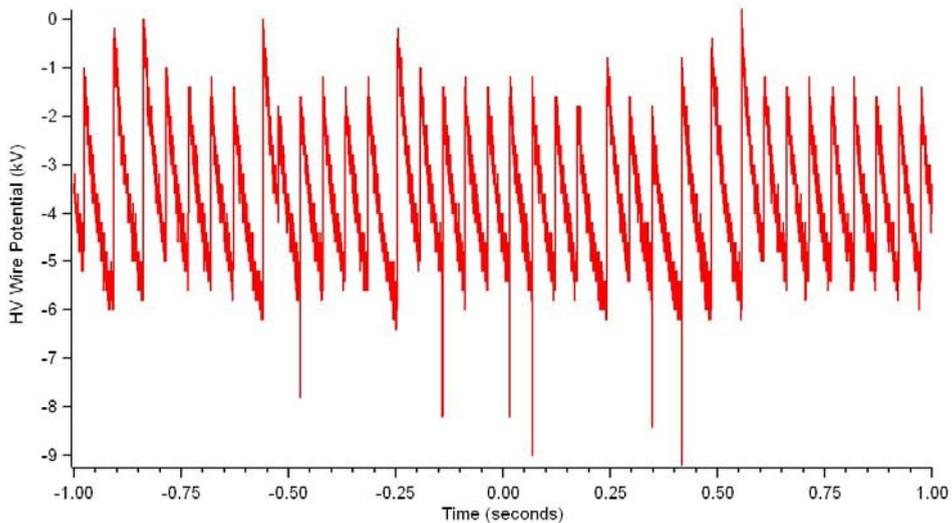
Fig. 7. Sample waveform delivered to the EP from both the Rotating Spark Gap and application of a HV DC offset.
