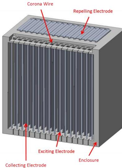
**Fig. 4.** Outline of the prototype of the new EAC.
