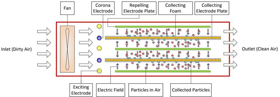
**Fig. 3.** Schematic diagram of the EAC with porous foam on the collecting electrodes.
