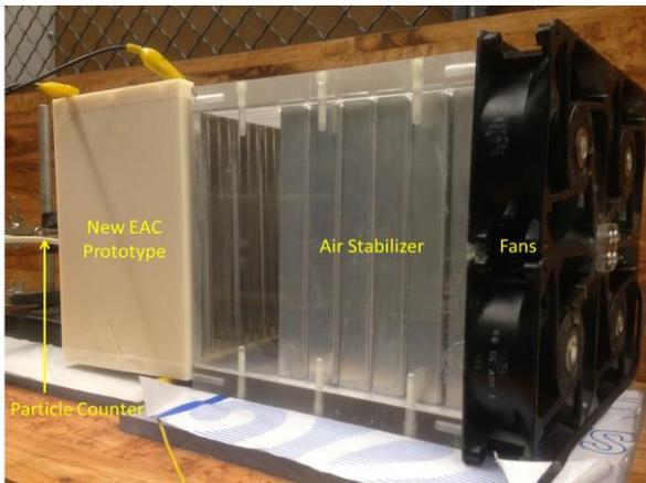
**Fig. 5.** Testing setup, including fans, air stabilizer, new EAC prototype, and particle counter.
