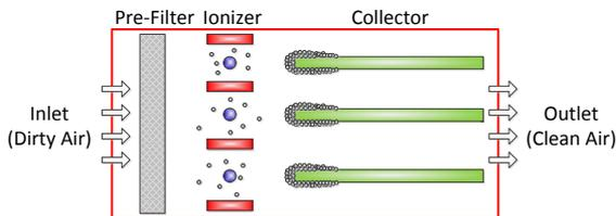
**Fig. 1.** Schematics of a traditional three stages EAC system.
