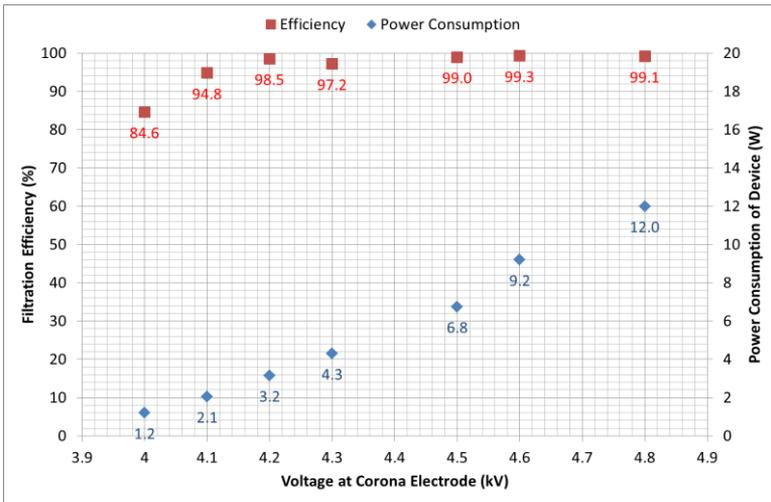
**Fig. 6.** Measurements of the filtration efficiency and the power consumption of the EAC itself at different corona electrode voltages. The particle diameter we focused on was 0.3  $\mu\text{m}$  to 5.0  $\mu\text{m}$ . The air velocity was 500 ft/min. The voltage at repelling electrode was 15 kV.
