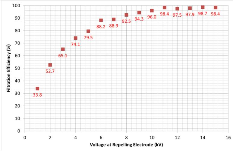
**Fig. 7.** Measurements of the filtration efficiency at different repelling electrode voltages. The particle diameter we focused on was 0.3 to 5.0 micrometers. The air velocity was 500 ft/min. The voltage at the corona electrode was 5 kV.
