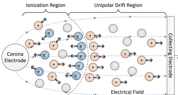
**Fig. 2.** Model of positive discharging. There are two regions between the corona and collecting electrodes. The ionization region, or corona plasma region, is formed and surrounds the corona electrode. The drift region is the region between the ionization boundary and the collecting electrode.
