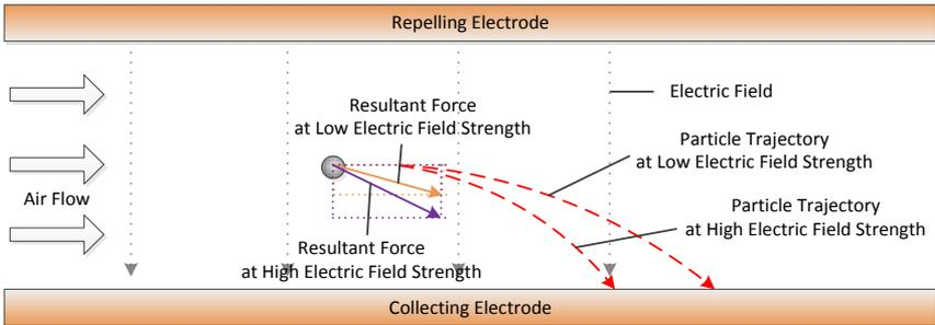
**Fig. 8.** Particle trajectories with high and low electric field strength. Not drawn to scale.
