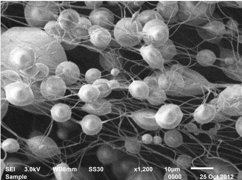
Fig. 2 SEM image of concurrent electrospaying (EFH1 ferrofluid) and PVA electrospinning (8% PVA water solution): +20kV PVA electrospinning, -6 kV ferrofluid electrospay, gap distance 5cm.
