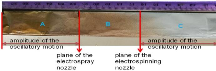
Fig.3 Photo of the collector's tin foil used for deposition.
