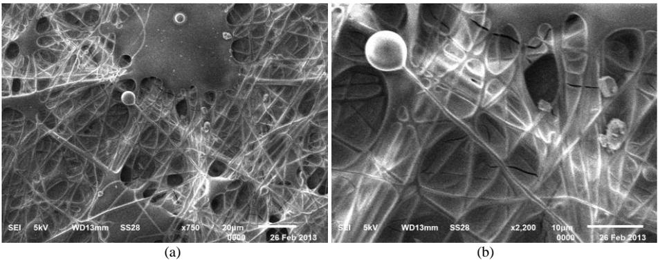
Fig. 4 Typical deposition layer: SEM images of concurrent electro spraying and electro spinning using a linearly oscillating collector
