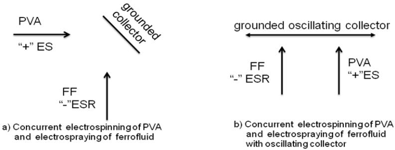
FF – ferrofluid; ES - electrospinning; ESR – electrospaying; PVA - polyvinyl alcohol
