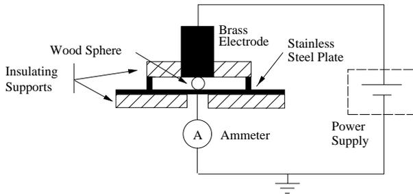
Fig. 3. Measurement of resistance of wood sample
