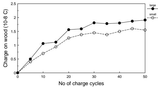
Fig. 7. Charge acquired by different sizes of hardwood spheres vs number of charging cycles
