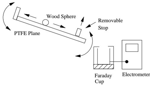
Fig. 1. Experimental setup for charging of wood sphere on PTFE platform
