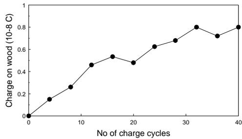
Fig. 5. Charge acquired by hardwood sphere vs number of charging cycles; no curve fitting
