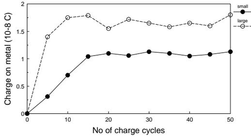
Fig. 9. Charge acquired by chrome plated steel and stainless steel spheres vs number of charging cycles
