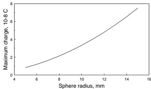
Fig. 10. Maximum charge on a conducting sphere vs sphere radius
