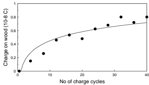
Fig. 4. Charge acquired by hardwood sphere vs number of charging cycles; data curve fitted
