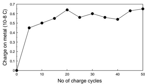
Fig. 8. Charge acquired by chrome plated steel sphere vs number of charging cycles
