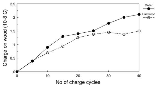
Fig. 6. Charge acquired by hardwood and softwood spheres vs number of charging cycles
