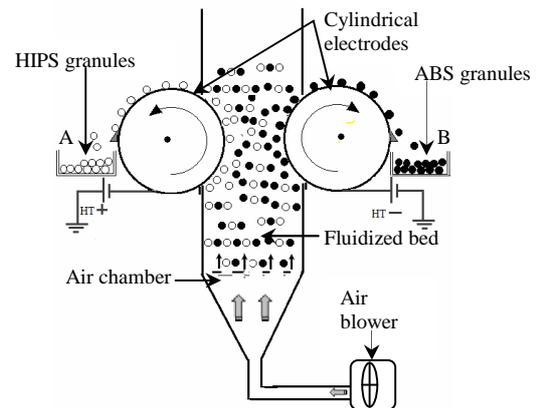
Fig. 1. Schematic representation of the new tribo-aero-electrostatic separation process.
