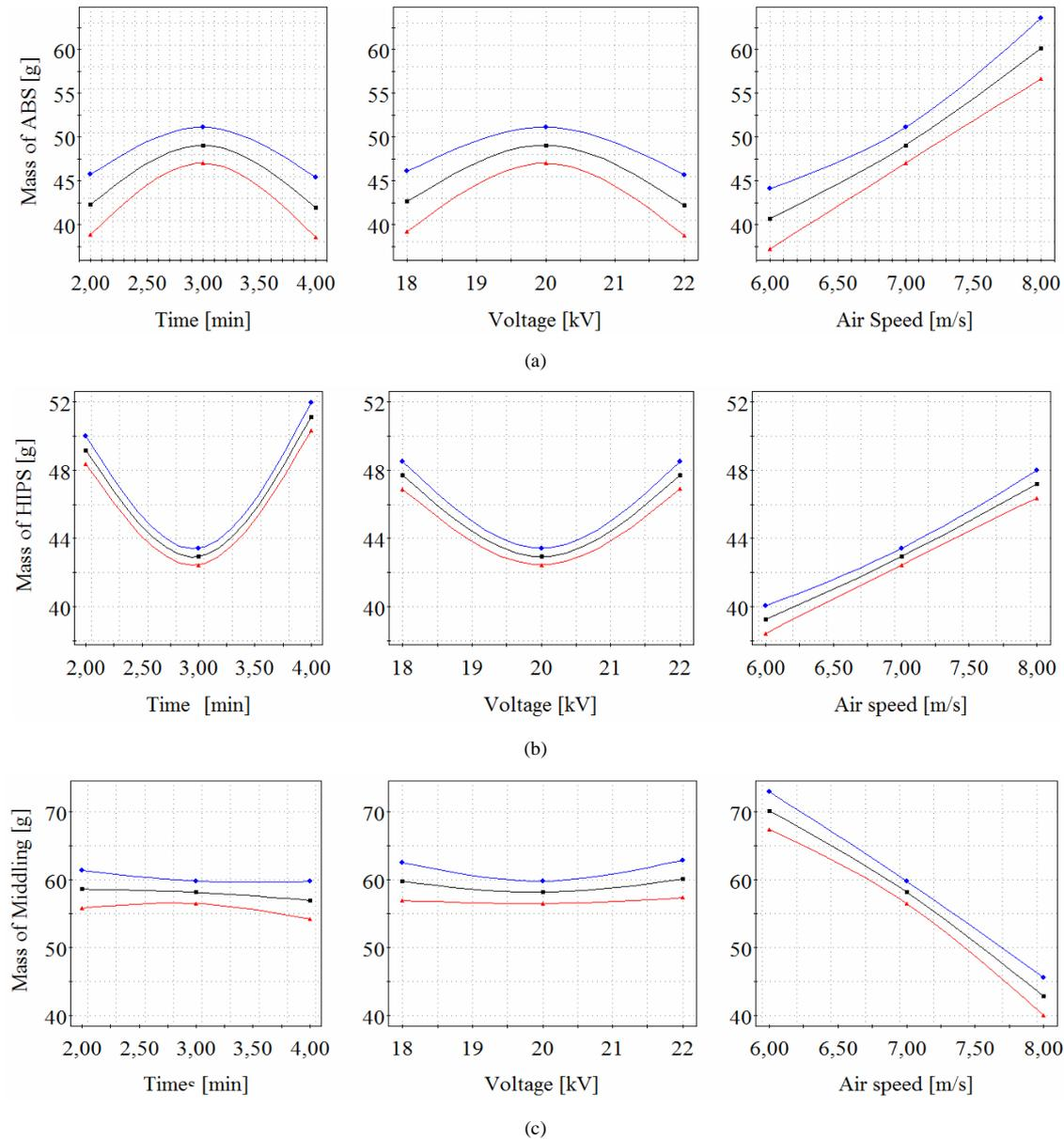
Fig. 7. MODDE-predicted masses of ABS (a) HIPS (b), and middling (c) as function of the duration  $T$ , the high-voltage  $U$ , and the air speed  $v$ . In each case, the other variables are maintained constant and equal to their central values  $T = 3$  min,  $U = 20$  kV, and  $v = 7$  m/s. The upper and lower curve on each graph indicate the limits of the 95% confidence level interval
