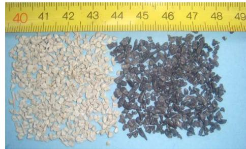
Fig. 4. Aspect and size of the granular materials (white: ABS; grey: HIPS).
