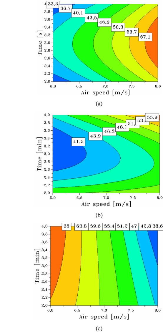
Fig. 6. MODDE 5.0 – computed equal response contours of ABS (a), HIPS (b) and Middling (c) masses for  $U = 18$  kV.
