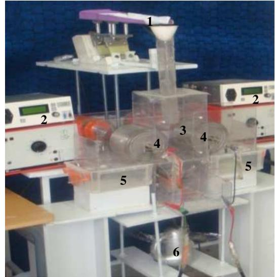
Fig. 3. Photograph of the laboratory tribo-aero-electrostatic separator 1: Vibratory feeder; 2: DC high-voltage supply; 3: Separation chamber; 4: Roll electrodes; 5: Collecting boxes; 6: Blower.
