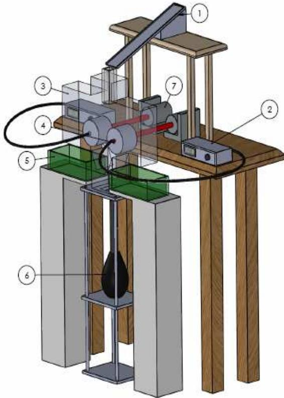
Fig. 2. Schematic representation of the modified tribo-aero-electrostatic separator; 1: Vibratory feeder; 2: DC high-voltage supplies; 3: Separation chamber; 4: Roll-type electrode; 5: Collecting box; 6: Blower, 7: Motor.
