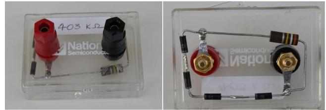
Fig. 12 Voltage limiting circuit
