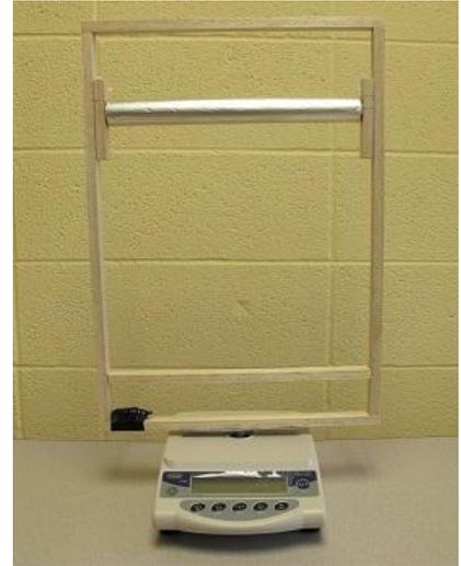
Fig. 9 Special design lifter attached to weighing scale
