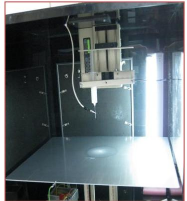
Fig. 1. (a) Electrospinning process and (b) experimental setup
