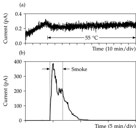
Figure 6. (a) Evolution of the signal at 55°C without smoke under 600 V. (b) Signal produced by smoke at 55°C under 600 V.
