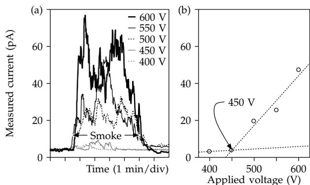
Figure 5. (a) Signals obtained at different applied voltage as a function of time when smoke enters the sensor. (b) Signal mean amplitude as a function of the applied voltage in presence of smoke.
