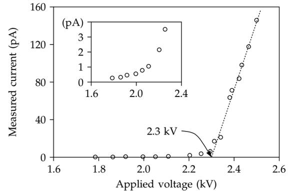
Figure 4. Measured current with the electrometer as a function of the applied voltage to the wire.
