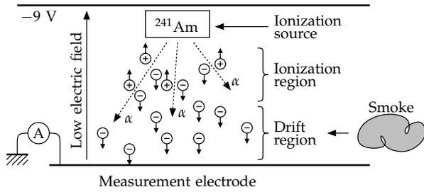
Figure 2. Principle of an ionic smoke sensor. In presence of smoke, much less charged particles reach the measurement electrode.
