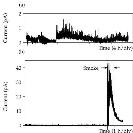
Figure 7. (a) Evolution of the signal at 40°C and 90% moisture without smoke under 600 V. (b) Signal produced by smoke at 40°C and 90% moisture under 600 V.
