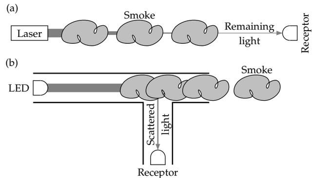
Figure 1. Principle of optical smoke sensors. (a) Operating mode for a detection over large areas. (b) Operating mode for a punctual detection. The source is often a light emitting diode (LED).
