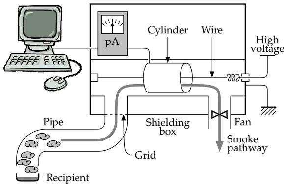
Figure 3. Experimental set-up. The sensor prototype is placed in a Faraday shielding box. It is fed with smoke driven by a fan from a pipe.
