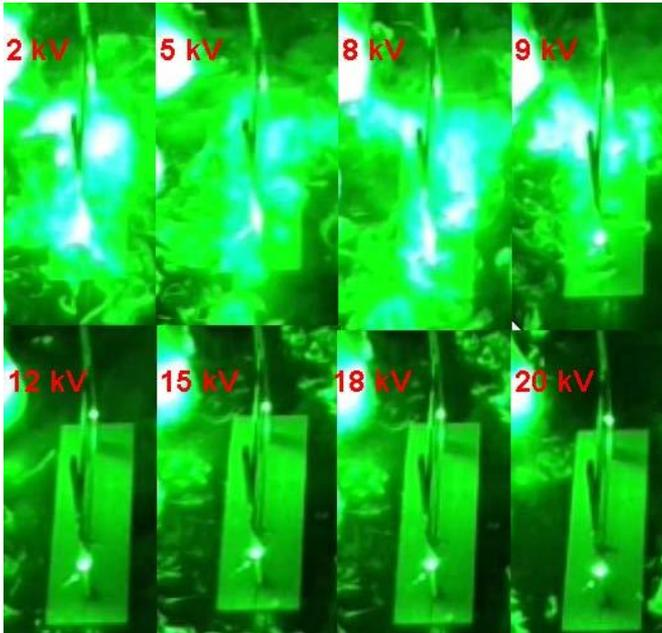
Fig. 3. Flow visualization: horizontal cross-section in the vertically generated ionic wind. The laser sheet is parallel to the base of the apparatus and at the lower level of the ground electrode.
