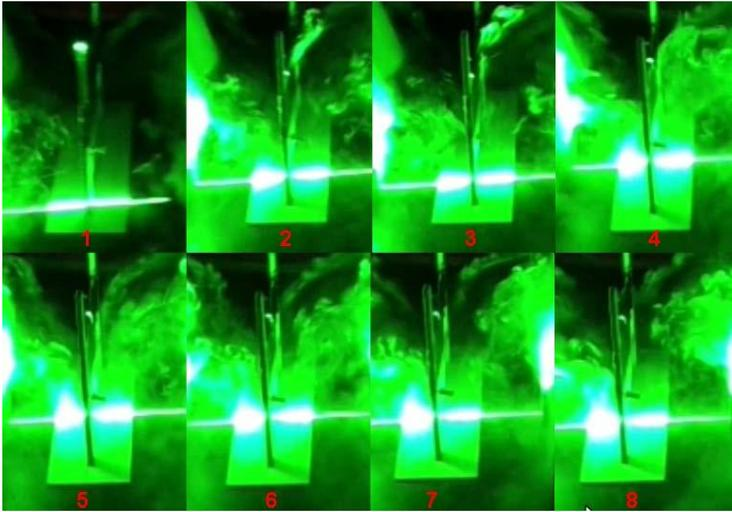
Fig. 4. Flow visualization: turbulent flow development in the corona wind. The image sequence was recorded within less than 1 second at 16.5 kV; the laser light comes vertically and perpendicular to the apparatus.
