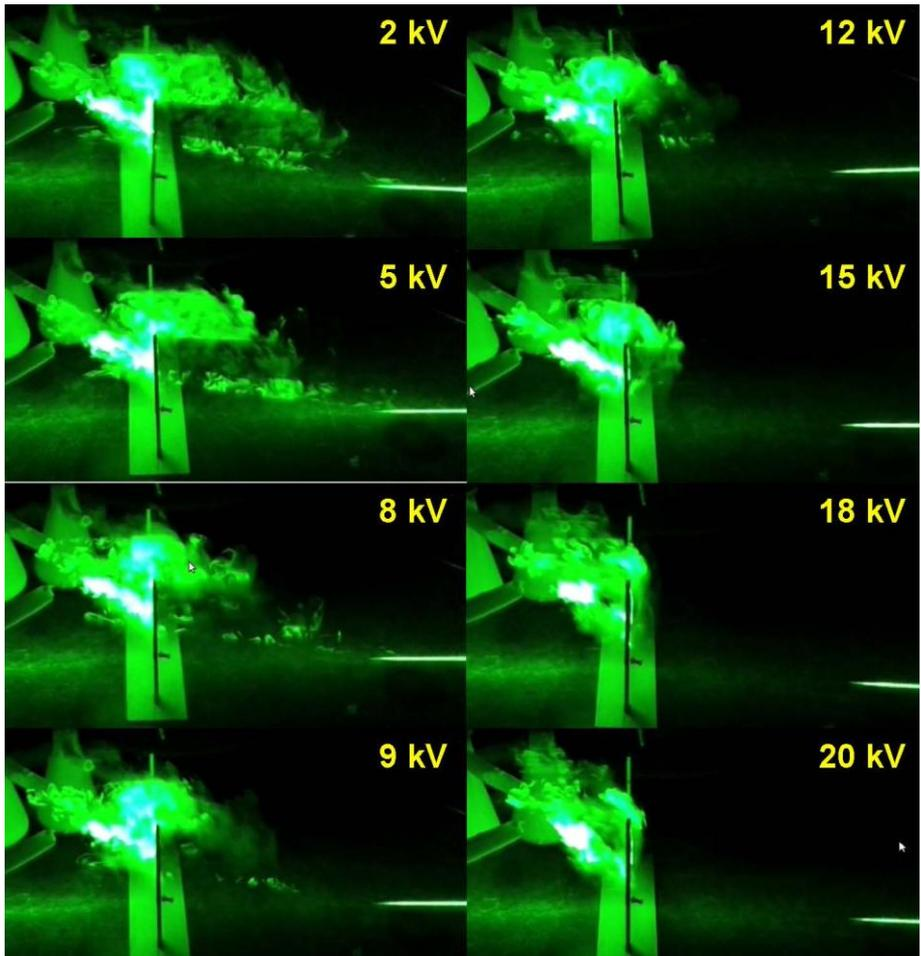
Fig. 2. Flow visualization: vertical cross-section of the turbulent flow of water vapors across the corona wind apparatus (laser light comes from the left and it is reflected back by a plane mirror on the right).
