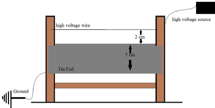
Fig. 1. Schematics of the apparatus (asymmetric capacitor).
