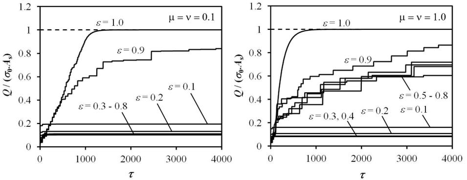
Fig. 5. Dimensionless charge vs. dimensionless time, for low friction (left) and high friction (right) cases. Charge calculated using the static capacitive charging model.
