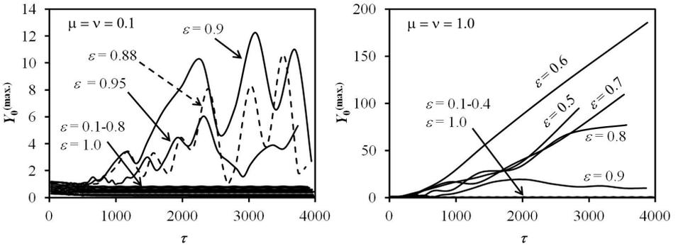
Fig. 4. Bounce amplitude vs. dimensionless time, for low friction (left) and high friction (right) cases. For  $\varepsilon = 0.1-0.4$  and  $\varepsilon = 1.0$ ,  $Y_0^{(\max.)} \approx 1$ .
