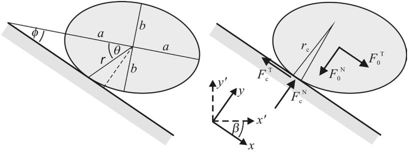
Fig. 1. Schematic of a two-dimensional elliptical particle in contact with a tilted surface, showing the coordinate axes, the important geometric quantities, and the forces on the particle.
