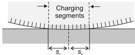
Fig. 2. Model contact between the particle and the plate. Charge is only transferred to those boundary segments that are in contact with the plate at any given time.
