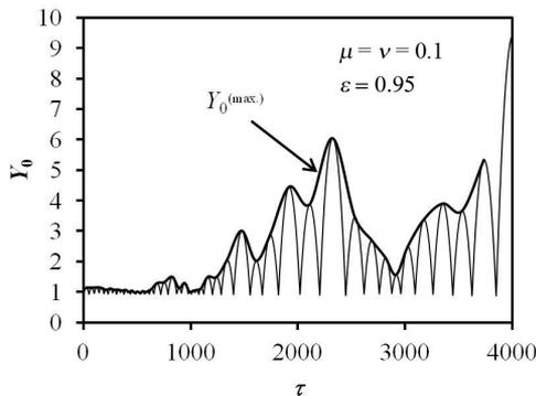
Fig. 3. The bouncing amplitude  $Y_0^{(\max.)}$  is obtained by taking the upper envelope of the normal particle-plate distance,  $Y_0$ .
