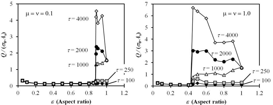
Fig. 8. Dimensionless charge vs. roundness ratio, for low friction (left) and high friction (right) cases, at various times. Charge calculated using the sliding contact charging model.
