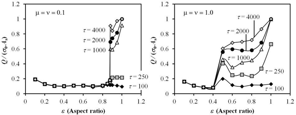
Fig. 6. Dimensionless charge vs. roundness ratio, for low friction (left) and high friction (right) cases, at various times. Charge calculated using the static capacitive charging model.
