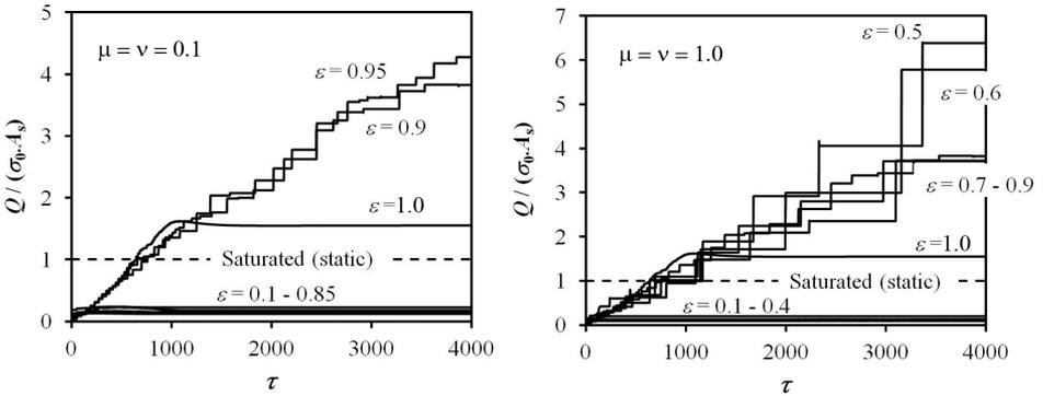
Fig. 7. Dimensionless charge vs. dimensionless time, for low friction (left) and high friction (right) cases. Charge calculated using the sliding contact charging model.
