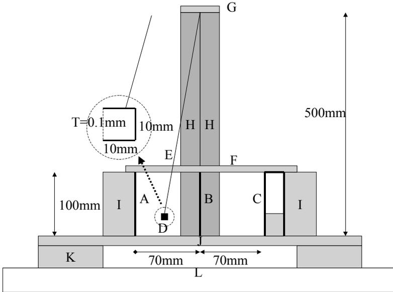
Fig. 15. Front view of the experiment instrument of the new electrostatic generator
