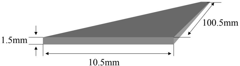
Fig. 2. The element plate that was used to compose all 19 conductors.
