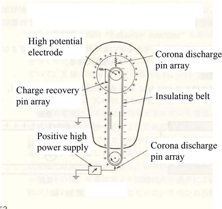
Fig. 13. Schematic layout of the Van de Graaff electrostatic generator [7]
