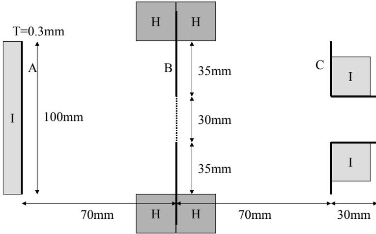
Fig. 17. Plane view of the experiment instrument of the new electrostatic generator
