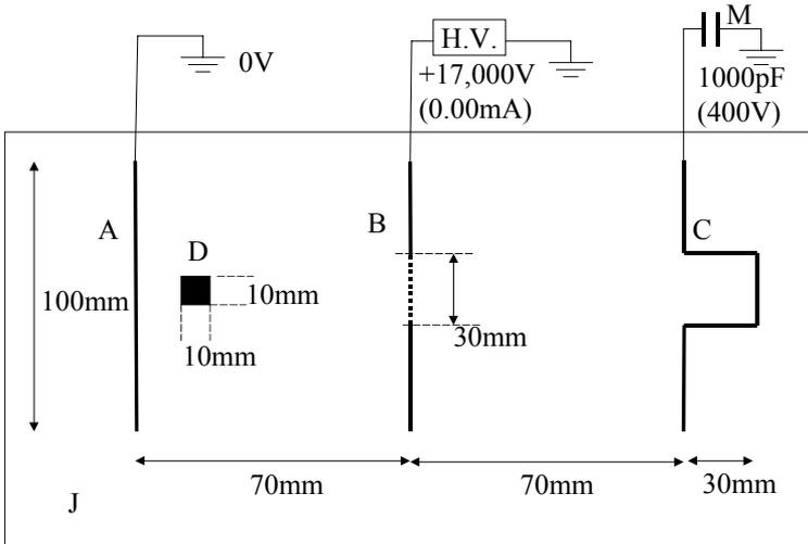
Fig. 18. Electric circuit of the experiment instrument of the new electrostatic generator
