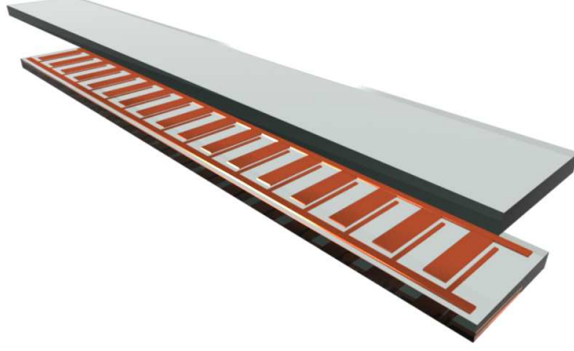
Fig. 1. The asymmetric arrangement of AC electroosmotic pumps
