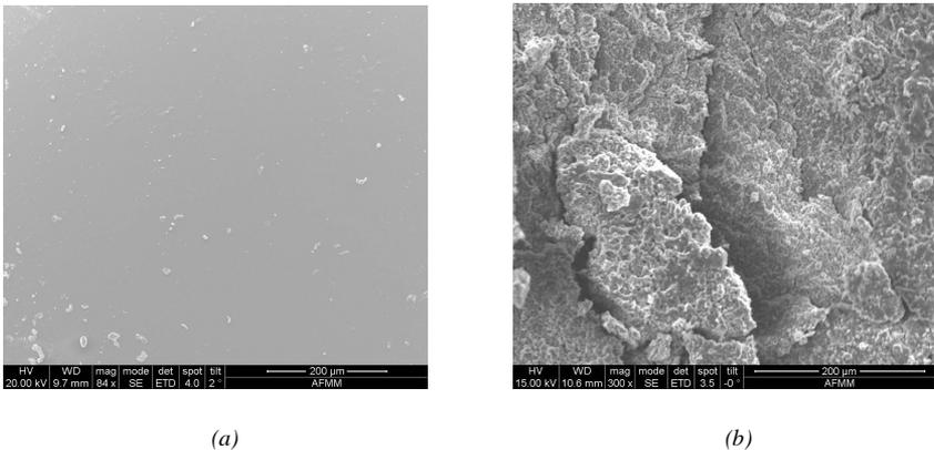
Fig. 5. SEM images with 200 um (a) fresh and (b) treated sample of silicon rubber
