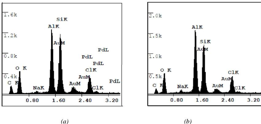
Fig. 6. EDAX analysis plots where x-axis is dispersive energy and y-axis is the X-ray counts where (a) is before treatment (b) after treatment
