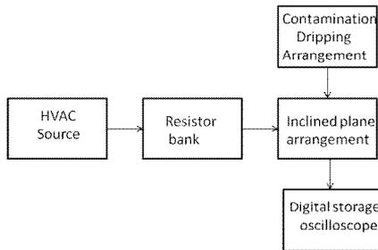
Fig. 1. Block diagram of experimental set up
