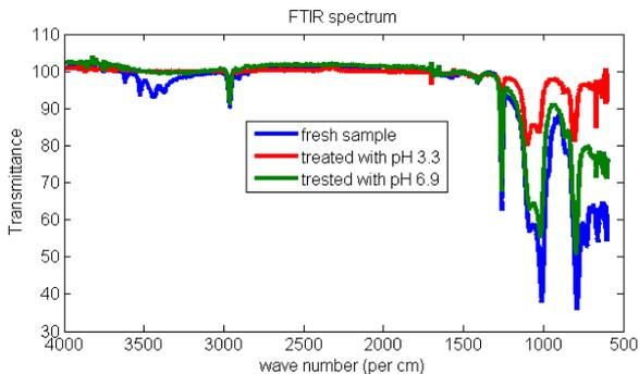
Fig. 7. FTIR spectrum comparing the fresh and treated samples with fresh and treated sample with pH 3.3 and pH 6.9
