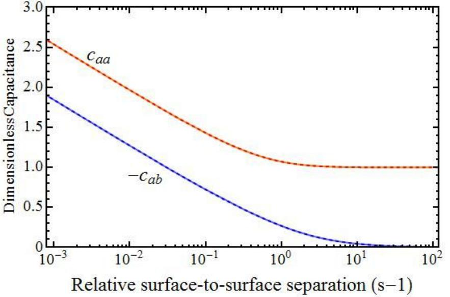
Fig. 2. The dimensionless capacitance coefficients for two equal-sized spheres are plotted versus their relative surface-to-surface separation  $s - 1$ . The solid lines are the exact results in Equation 2 and the dashed lines are the approximations obtained by substituting Equation 7 into Equation 4. The relative error in the approximations is only 0.05% and the two approximation curves lie on top of their corresponding exact results.
