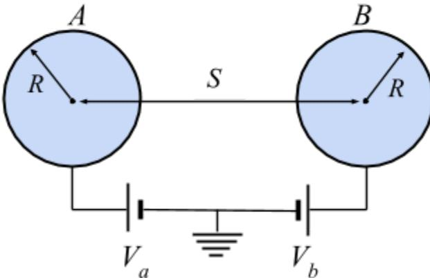
Fig. 1. Basic geometry of our setup. The charge on each sphere depends upon the applied voltages  $V_a$  and  $V_b$ , and the distance  $S$  between them.
