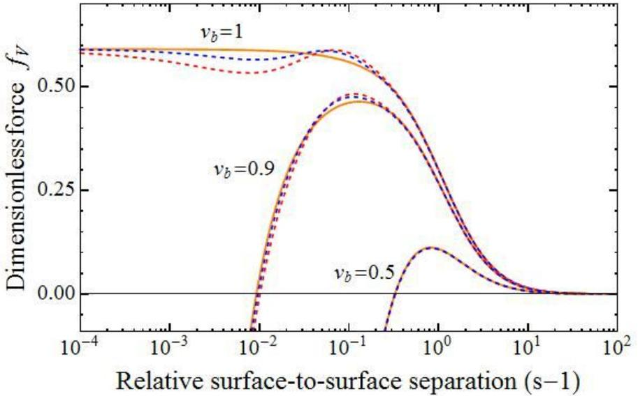
Fig. 3. The dimensionless force between two equal-sized spheres is plotted versus their relative surface-to-surface separation  $s - 1$  for several different voltage ratios. The solid lines are the exact results and the red and blue dashed lines are the approximations obtained by substituting Equations 7 and 8 respectively into Equation 4.
