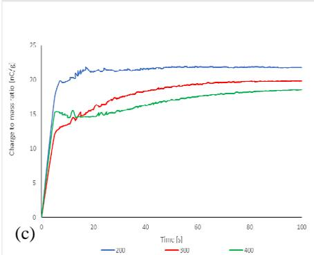
Fig. 4. Mass (a), charge (b) and charge/mass ratio (c) vs. time, for the ABS product recovered from 200 g, 300 g and 400 g samples of a granular mixture composed of 50% ABS and 50% PS (air flow rate:  $n = 6.4 \text{ m}^3/\text{h}$ ; applied high voltage:  $U = \pm 8 \text{ kV}$ ; rotating speed of the disk electrodes:  $v = 30 \text{ rpm}$ ; and duration of the pre-charging  $t_c = 0 \text{ s}$ )
