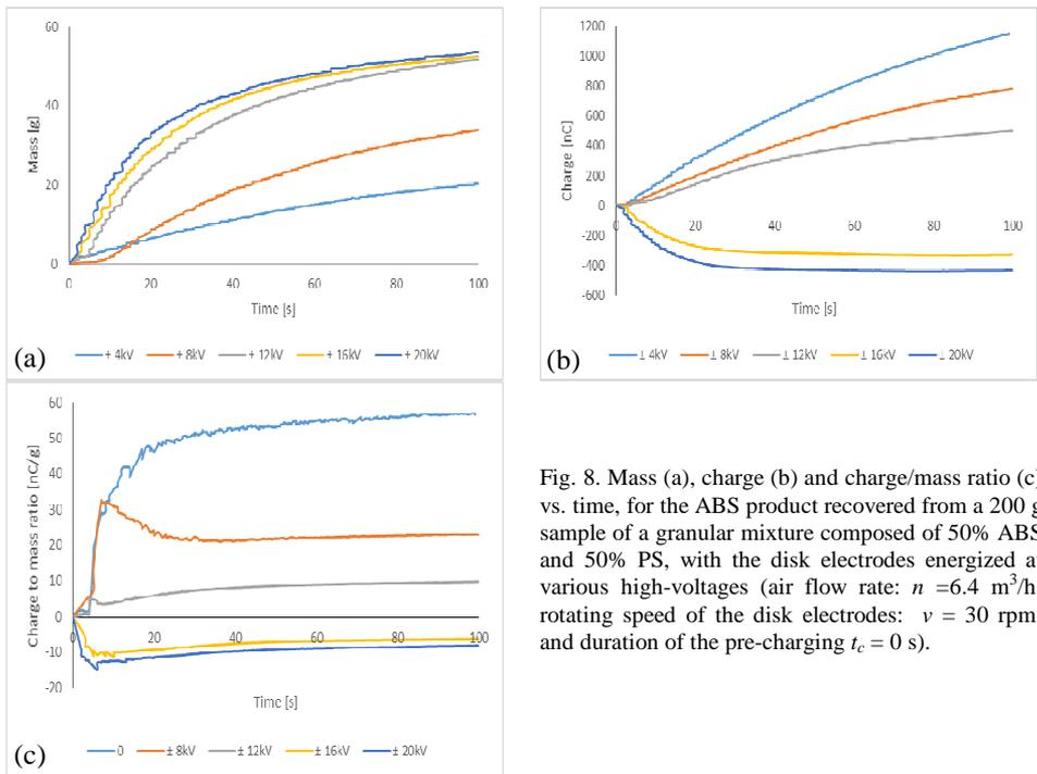
Fig. 8. Mass (a), charge (b) and charge/mass ratio (c) vs. time, for the ABS product recovered from a 200 g sample of a granular mixture composed of 50% ABS and 50% PS, with the disk electrodes energized at various high-voltages (air flow rate:  $n = 6.4 \text{ m}^3/\text{h}$ ; rotating speed of the disk electrodes:  $v = 30 \text{ rpm}$ ; and duration of the pre-charging  $t_c = 0 \text{ s}$ ).
