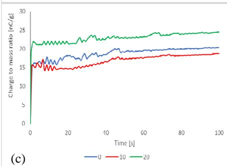
Fig. 5. Mass (a), charge (b) and charge/mass ratio (c) vs. time, for the ABS product recovered from a 200 g sample of a granular mixture composed of 50% ABS and 50% PS, pre-charged for three charge durations  $t_c = 0 \text{ s}$ ,  $10 \text{ s}$  and  $20 \text{ s}$  (air flow rate:  $n = 6.4 \text{ m}^3/\text{h}$ ; applied high voltage:  $U = \pm 8 \text{ kV}$ ; rotating speed of the disk electrodes:  $v = 30 \text{ rpm}$ ).
