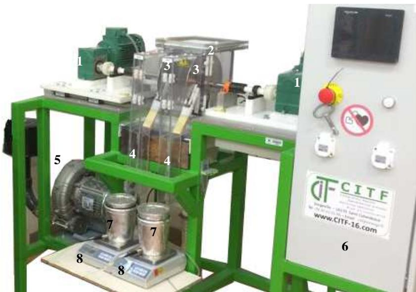
Fig. 1. Two-rotating-disks-type tribo-aero-electrostatic separator;
