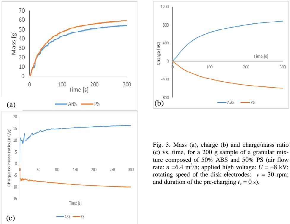
Fig. 3. Mass (a), charge (b) and charge/mass ratio (c) vs. time, for a 200 g sample of a granular mixture composed of 50% ABS and 50% PS (air flow rate:  $n = 6.4 \text{ m}^3/\text{h}$ ; applied high voltage:  $U = \pm 8 \text{ kV}$ ; rotating speed of the disk electrodes:  $v = 30 \text{ rpm}$ ; and duration of the pre-charging  $t_c = 0 \text{ s}$ ).
