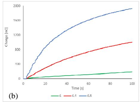
Fig. 6. Mass (a), charge (b) and charge/mass ratio (c) vs. time, for the ABS product recovered from a 200 g sample of a granular mixture composed of 50% ABS and 50% PS, charged for three air flow-rates  $n = 6 \text{ m}^3/\text{h}$ ,  $6.4 \text{ m}^3/\text{h}$  and  $6.8 \text{ m}^3/\text{h}$  (applied high voltage:  $U = \pm 8 \text{ kV}$ ; rotating speed of the disk electrodes:  $v = 30 \text{ rpm}$ ; and duration of the pre-charging  $t_c = 0 \text{ s}$ ).
