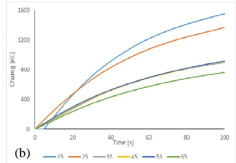
Fig. 7. Mass (a), charge (b) and charge/mass ratio (c) vs. time, for the ABS product recovered from a 200 g sample of a granular mixture composed of 50% ABS and 50% PS, with the disk electrodes rotating at various speeds (air flow rate:  $n = 6.4 \text{ m}^3/\text{h}$ ; applied high voltage:  $U = \pm 8 \text{ kV}$ ; and duration of the pre-charging  $t_c = 0 \text{ s}$ ).
