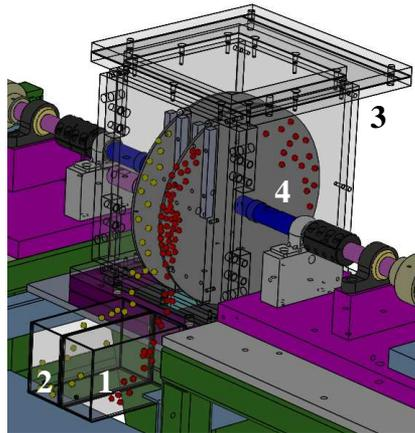
Fig. 2. Two-box collecting system of the laboratory two-rotating-disks-type tribo-aero-electrostatic separator; 1: Collecting box for positively-charged ABS particles; 2: Collecting box for negatively-charged PS particles; 3: Separation chamber, 4: Disks.
