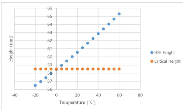
Fig. 11. Comparison between HFE heights and the critical height at different temperatures.
