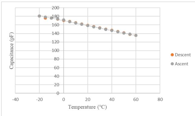
Fig. 4. Capacitance as a function of temperature.
