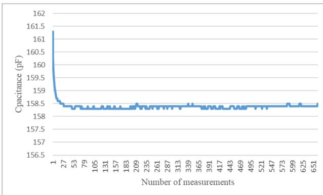
Fig. 2. The evolution of capacitance with time at  $20^{\circ}\text{C}$ .
