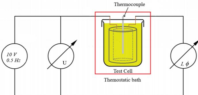
Fig. 1. Schematic view of the test cell used for the dielectric measurements.
