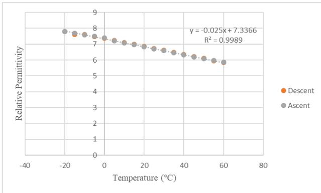
Fig. 6. Relative permittivity as a function of temperature.
