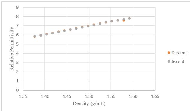
Fig. 7. Relative permittivity as a function of density.
