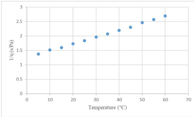
Fig. 12. Inverse of the dynamic viscosity as a function of temperature.
