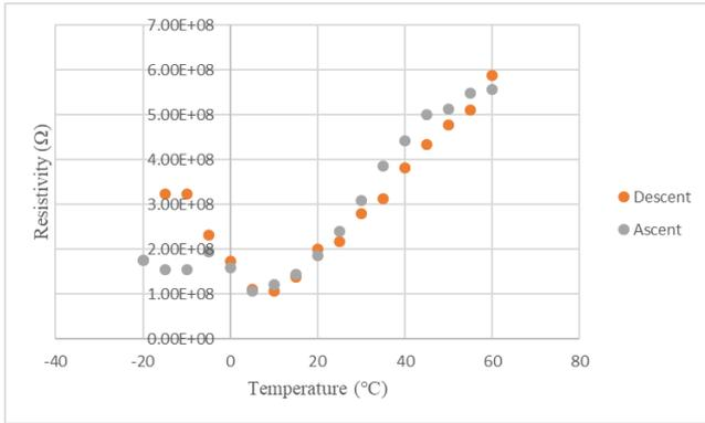
Fig. 10. Resistivity as a function of temperature.
