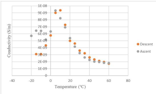
Fig. 9. Conductivity as a function of temperature.
