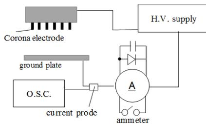
Figure 2 Measuring circuit
