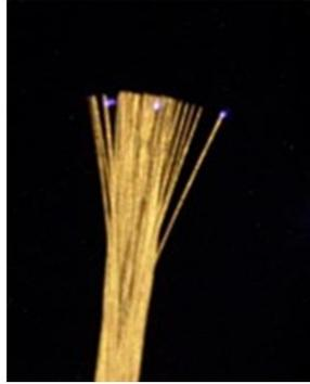
Figure 1 Bundle of fine metal fibers
