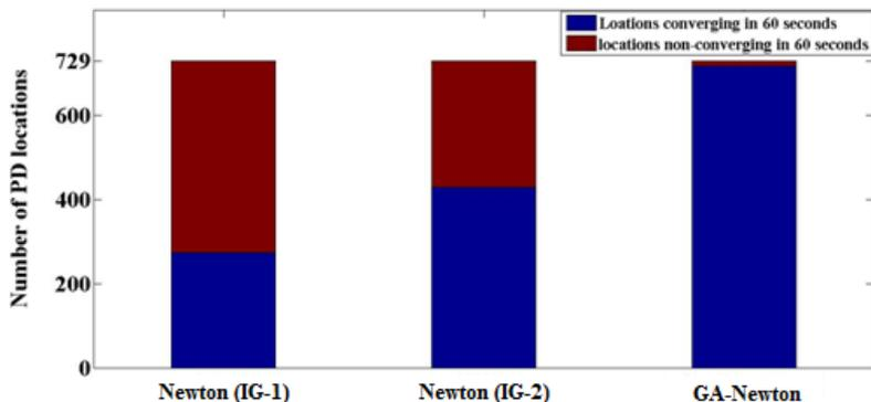
Fig. 2. Comparison of number of PD sources converging or non-converging within 60 seconds by using Newton's method with different initial guesses and GA-Newton method
