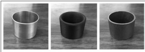
Fig. 3. Collector materials. Shown from left to right are aluminum, 3-D printed graphite/PLA, and copper collectors tested.
