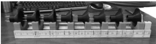
Fig. 4. Emitter/Collector pairs. Conical collectors are shown with integral emitters. In this configuration, every other device would be charged negative with remaining units charged positively giving alternating positive and negative coronas.
