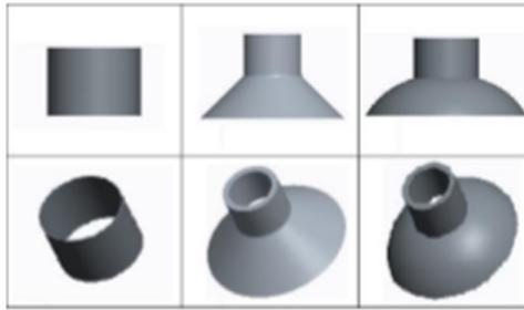
Fig. 2. Collector Shapes. Shown from left to right are cylindrical, conical, and parabolic profile collectors tested. Only cylindrical and conical were compared in the DOE.
