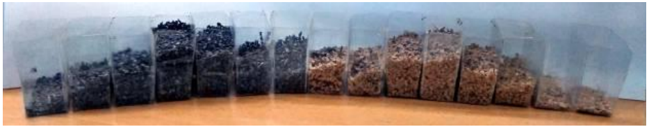
Fig. 6. Products recovered in the collector cells (diameters of particles 1.4 \text{ mm} < \varnothing < 2.8 \text{ mm} )
