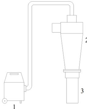
Fig. 1. Components of the turbulent tribocharger. (1) Air vacuum pump, (2) cyclone, (3) cylindrical container.
