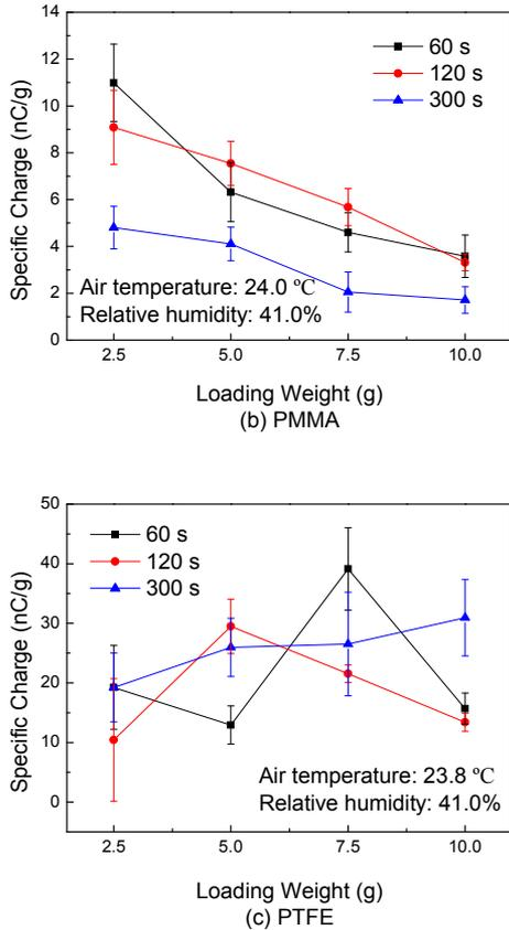
Fig. 5. Influence of granule loading weight on specific charge in different containers.
