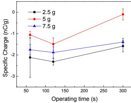
Fig. 4. Effect of operating time on specific charge in copper container (Air temperature: 23.6°C, relative humidity: 10.6%).
