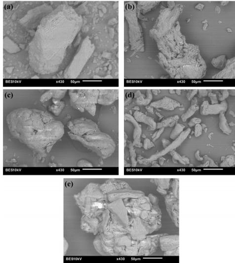
Fig. 3. Scanning electron micrographs of the pharmaceutical powders. (a) Lactose monohydrate (LMH), (b) Microcrystalline Cellulose (MCC), (c) Hydroxypropyl Methylcellulose (HPMC), (d) Croscarmellose Sodium (CCS), (e) dry granule sample
