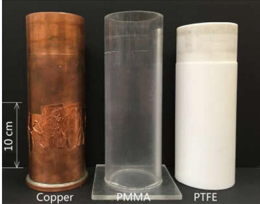
Fig. 2. Cylindrical containers made of copper, PMMA, and PTFE.
