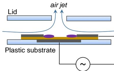
Fig. 1. Illustration showing ionic wind air jet produced by ring electrode DBD.
