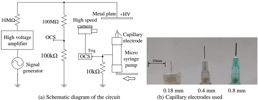
Fig. 1. Experimental circuit for observing corona discharge from a water droplet
