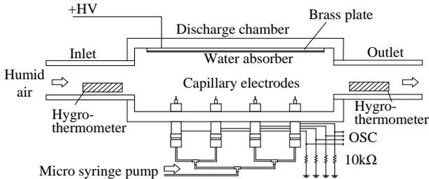
Fig. 2. Dehumidifier by charge droplet produced from corona discharge from four capillary electrodes.
