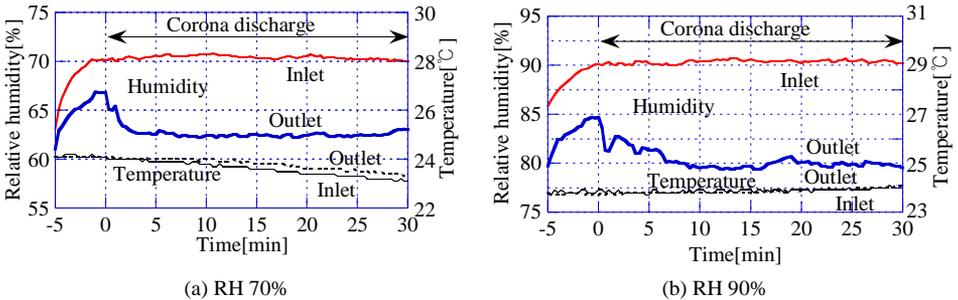
Fig. 4. Time variation of relative humidity of humid air into the discharge chamber.
