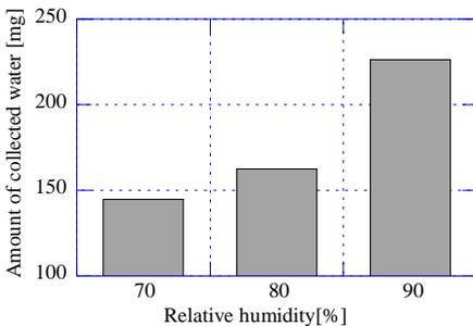
Fig. 5. Collected water contents from humid air by negative corona discharge from water droplets.
