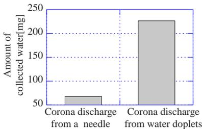
Fig. 8. Effect of the corona discharge on the amount of collected water.
