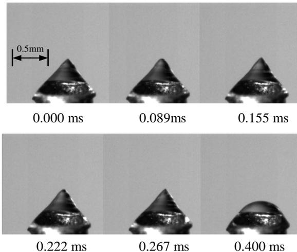
Fig. 6. Cone formation and disruption during corona discharge from a water droplet formed at 0.8 mm diameter capillary electrode.
