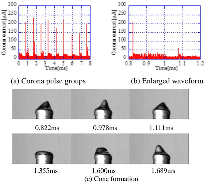
Fig. 3. Cone formation and disruption during corona discharge from a water droplet formed at 0.4 mm diameter capillary tube.
