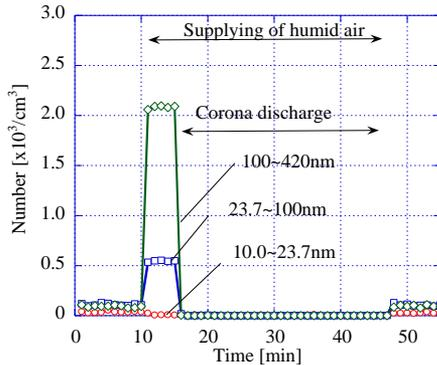
Fig.9. The time variation of the number of vapor particle in air with or without corona discharge.
