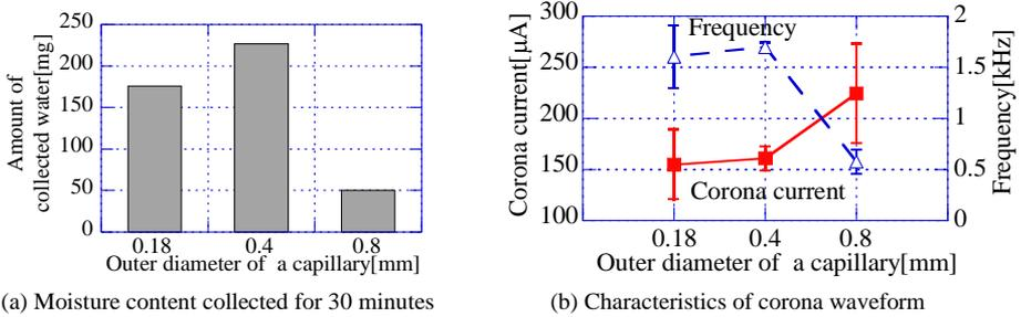
Fig. 7. Effect of the size of capillary electrode on collected water contents and the magnitude and occurrence frequency of disruption from a water droplet.
