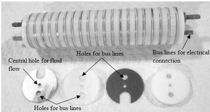
Fig. 2. Assembled EHD conduction pump with 20 electrode pairs and individual electrodes and spacers [21 and 22]
