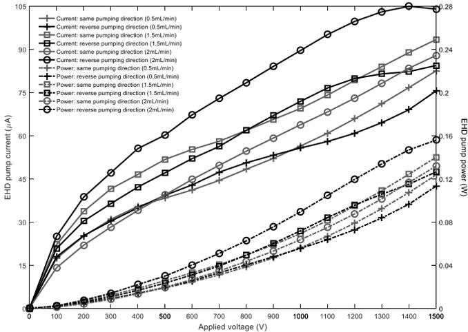
Fig. 8. Comparison of EHD pump current and power in the active branch between the two pumping direction configurations (0.5 mL/min, 1.5 mL/min and 2 mL/min cases)
