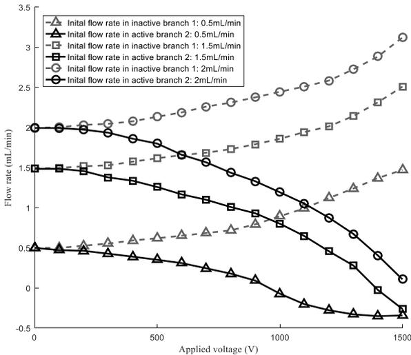
Fig. 3. Measured flow rates in both branches for the reverse EHD pumping direction configuration (0.5 mL/min, 1.5 mL/min, and 2 mL/min case)
