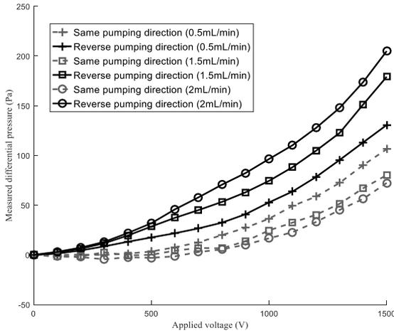
Fig. 7. Comparison of measured differential pressure across EHD conduction pumps in the active branch between the two pumping direction configurations (0.5 mL/min, 1.5 mL/min and 2 mL/min cases)
