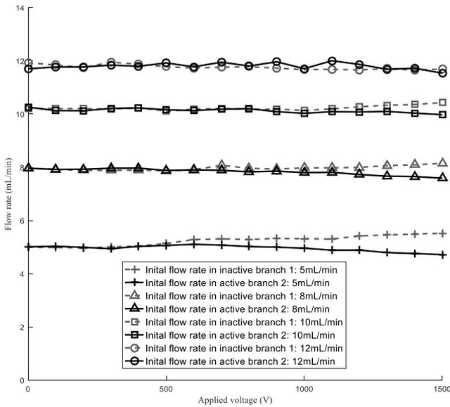
Fig. 4. Measured flow rates in both branches for the reverse EHD pumping direction configuration (5 mL/min, 8 mL/min, 10 mL/min and 12 mL/min case)
