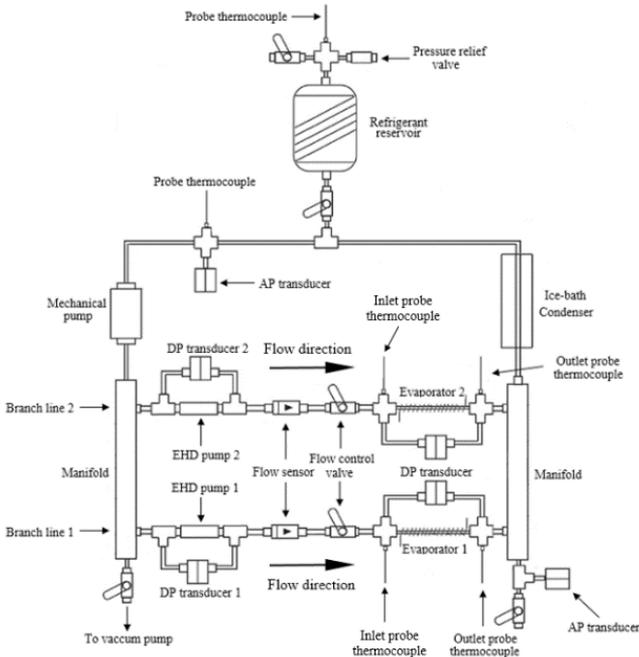
Fig. 1. EHD conduction pump driven liquid flow distribution control experimental setup
