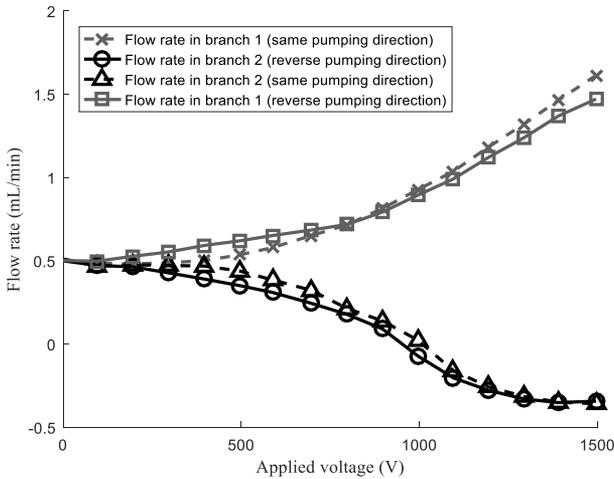
Fig. 5. Comparison of measured flow rates in both branches between the two pumping direction configurations (initially equal flow distribution of 0.5 mL/min in each branch)
