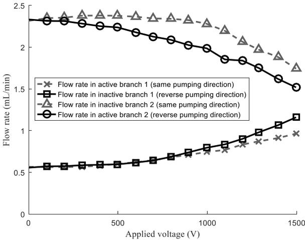
Fig. 10. Comparison of measured flow rates in both branches for the same pumping direction and the reverse pumping direction (initially maldistributed flow distribution of 0.6 mL/min and 2.3 mL/min)
