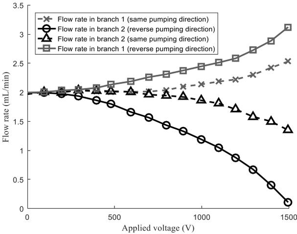
Fig. 6. Comparison of measured flow rates in both branches between the two pumping direction configurations (initially equal flow distribution of 2 mL/min in each branch)
