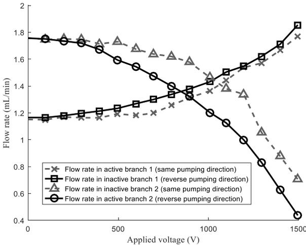
Fig. 9. Comparison of measured flow rates in both branches between the same pumping direction and the reverse pumping direction (initially maldistributed flow distribution of 1.15 mL/min and 1.75 mL/min)
